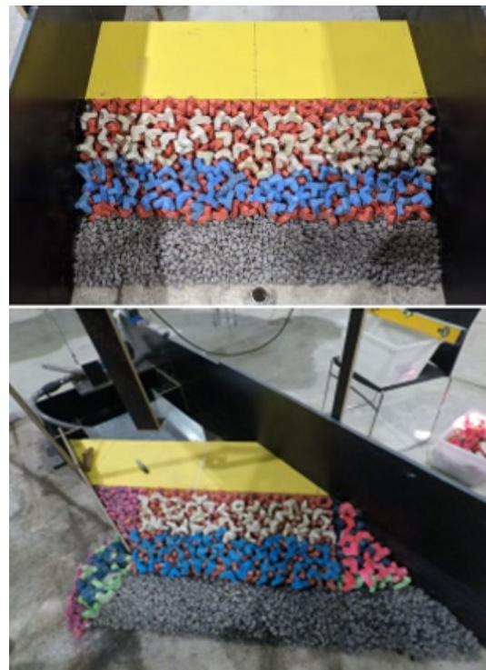
Figure 6: 2D Physical model tests were used to define site specific stability coefficients for waves approaching head on (top) and at 45^\circ (bottom).
