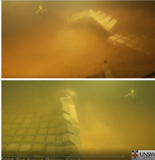
(a) Underwater video footage showing flapping of leading edge of ACMs
