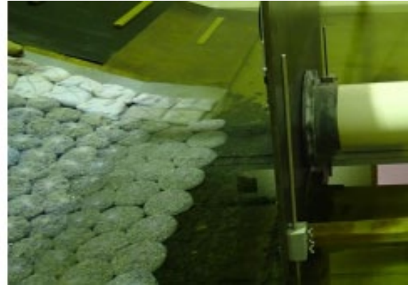
Figure 11 Rock bags on revetment slope in front of bow thruster setup
