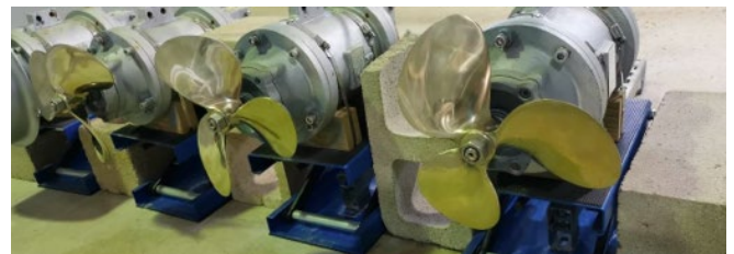
Figure 4 Four independently controlled propellers
