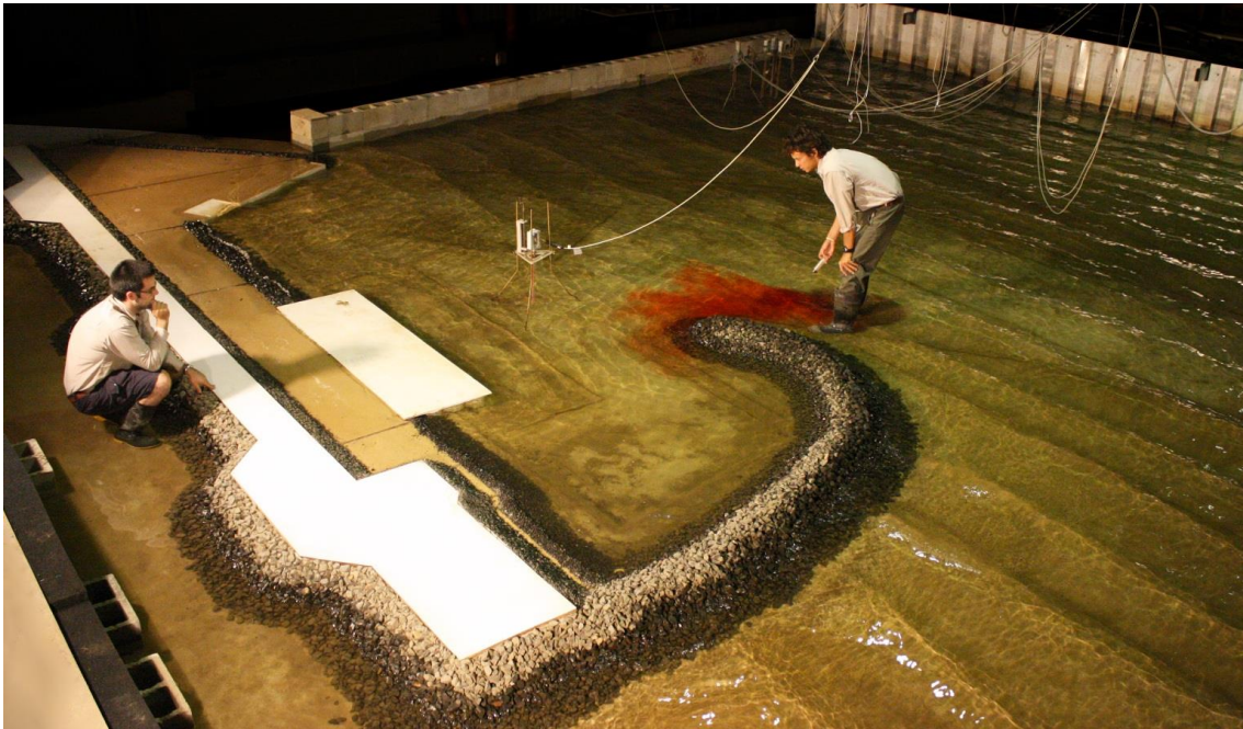
Physical modelling of Barrow Island LNG plant materials offload facility
