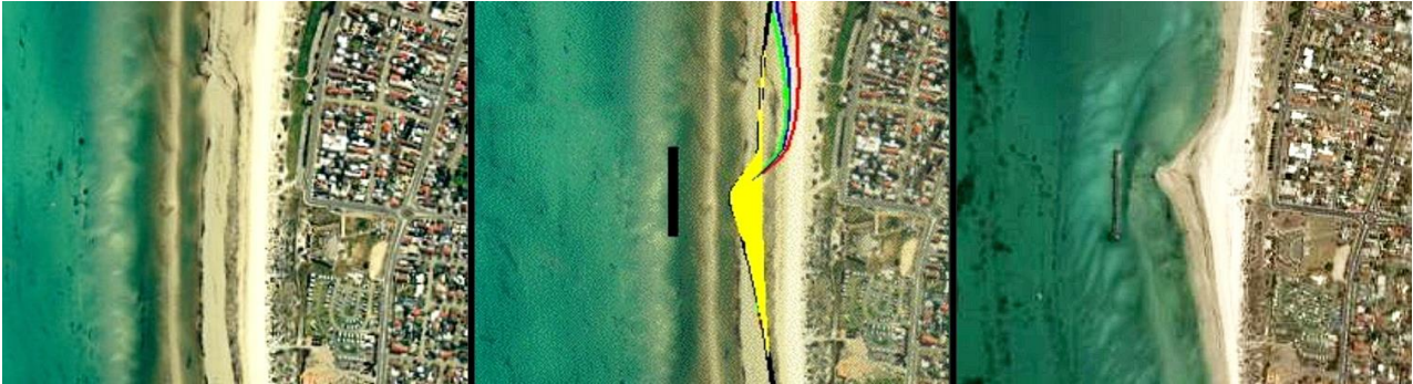
GENESIS Modelling for detailed design of Semaphore Park offshore breakwater (SA)
