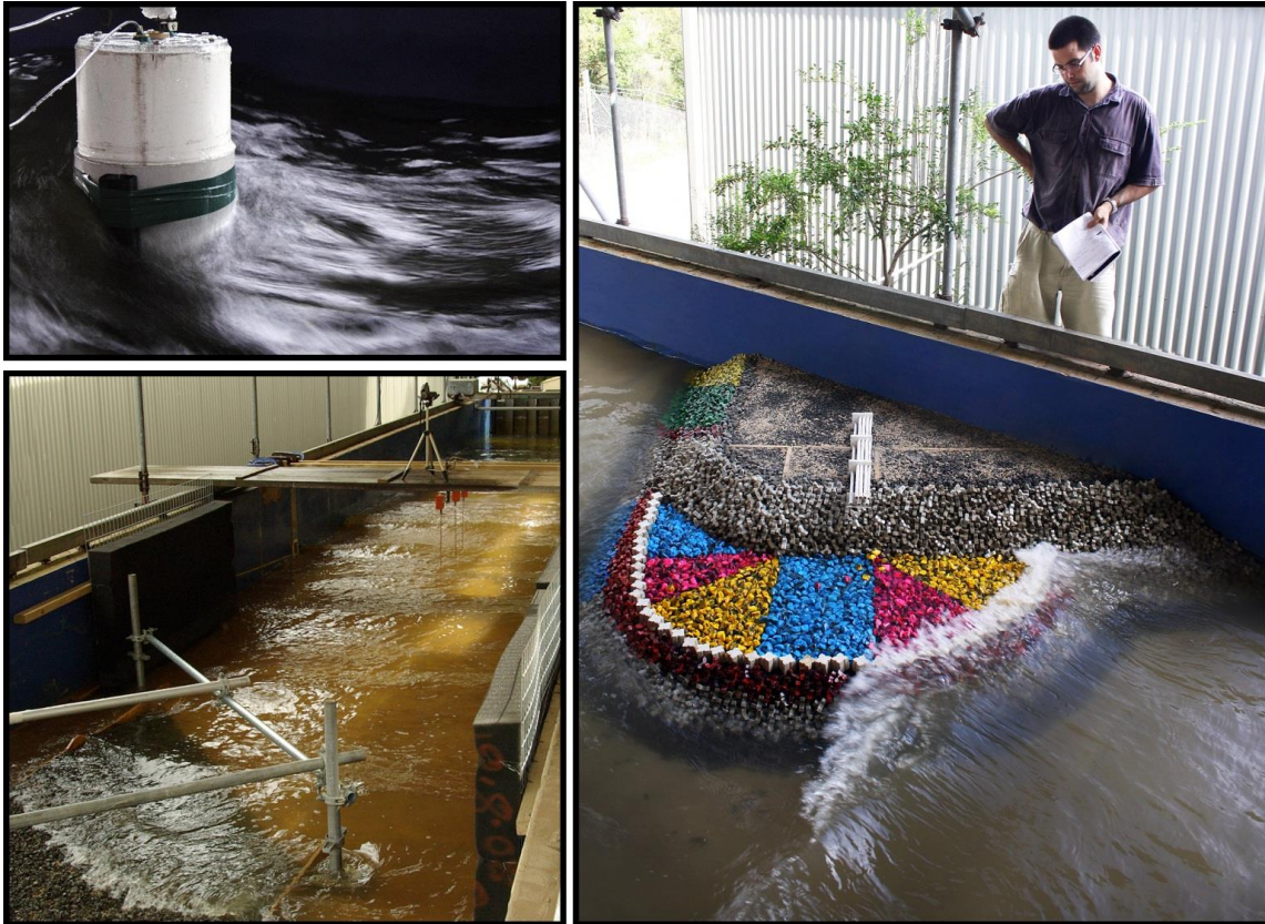
(Top left) Physical model testing of Oceanlinx Wave Energy System; (Bottom left, and right) Physical modelling of Barrow Island LNG plant materials offload facility
