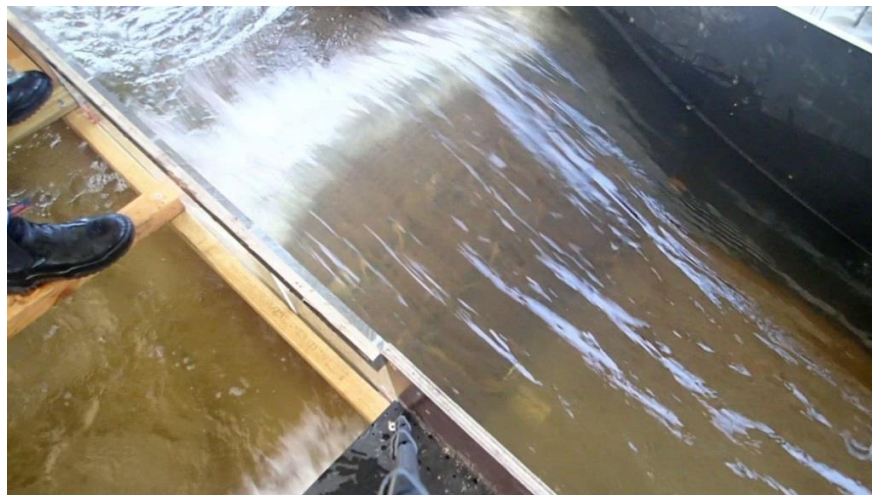
Figure 3: Oyster Shell Filled Bags Under Wave Attack in WRL's 3 m Wave Flume Note – Wave are Travelling from Right to Left
