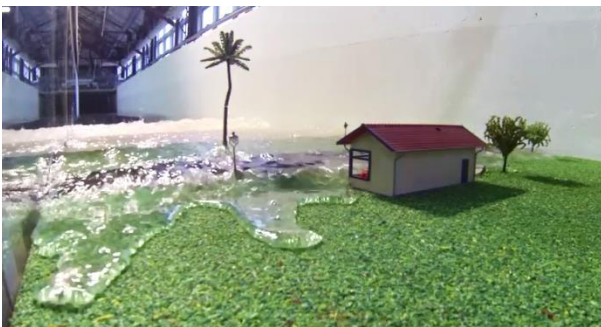
Physical model of reef overtopping during storm surge
