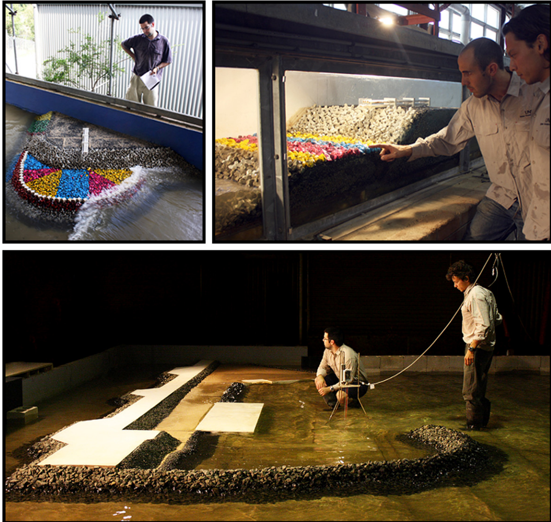
(Clockwise) Quasi-3D flume testing – 3 m wave flume; 2D flume testing – 1 m wave flume; 3D wave basin modelling
